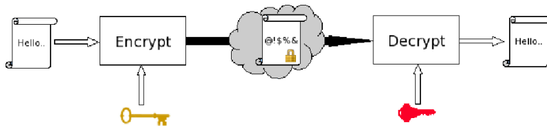
Figure 3.5: Schematic of an asymmetric encryption scheme
